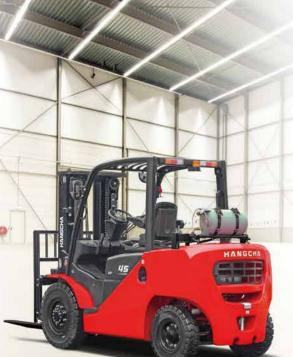
In developing the new XF Series, comfort and ease of operation is carefully considered, for example, to improve vibration levels, compound engine damper and full floating power train are adopted.
